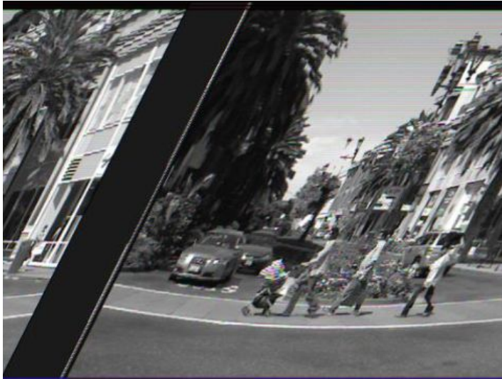
Example of a Fault in the Clock System
